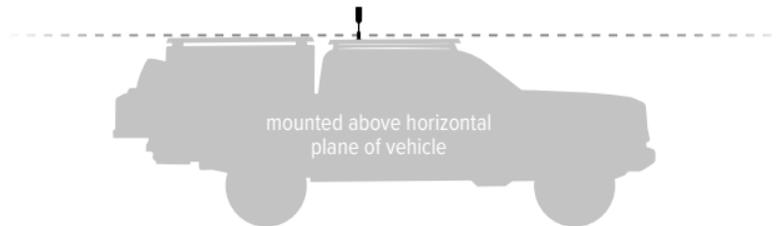
For best performance the outside antenna should be mounted above the horizontal plane of the vehicle and/or above other gear on top of the vehicle.
