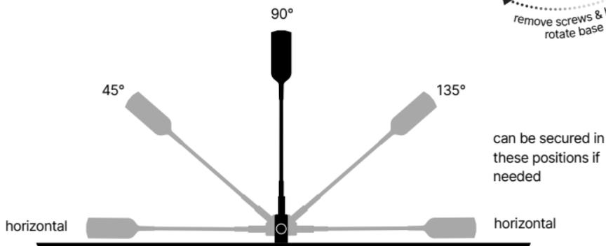
NOTE: System will only fully function with the antenna in the upright position.
