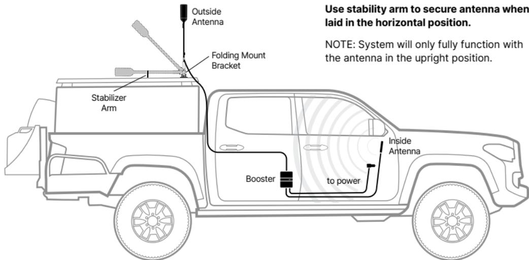
**Use stability arm to secure antenna when laid in the horizontal position.**
